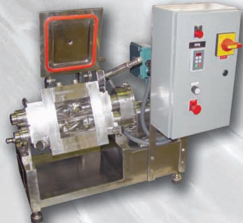
1 Liter Laboratory Mixer Supplied for the manufacture of Automotive Sealants
