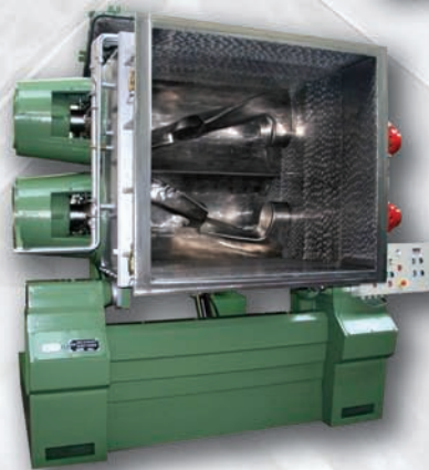
Rebuilt 1400 Liter Mixer Supplied for the manufacture of Silicone Products
