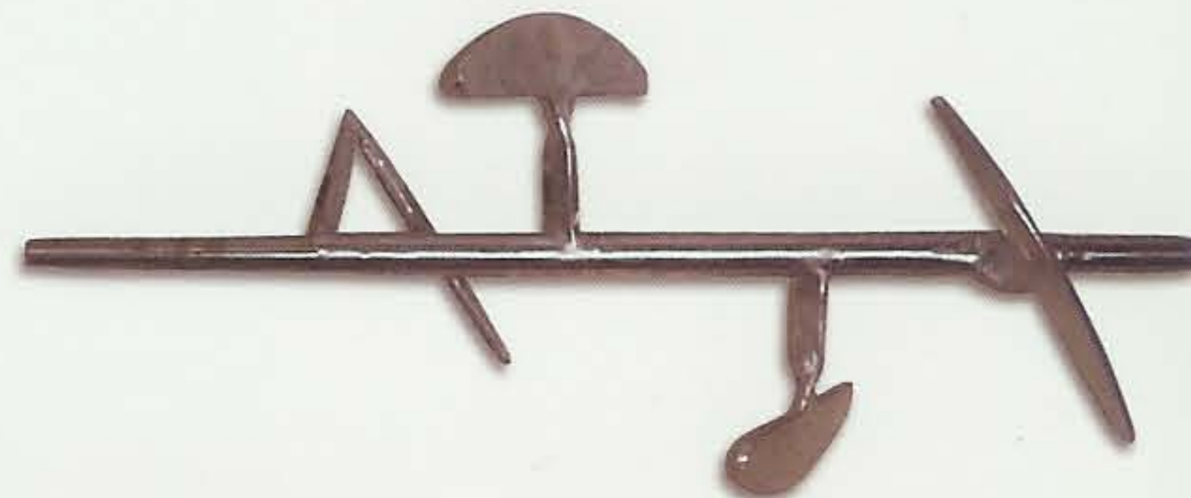
JAYGO JTB mixer interior shaft, with paddle type mixing elements.
