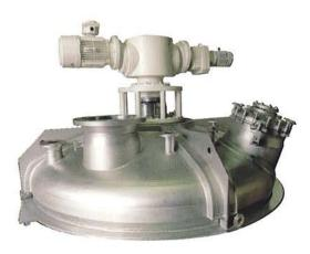
Special dam construction in main drive and orbit arm prevents contaminants or lubricants from entering the mixing vessel.
