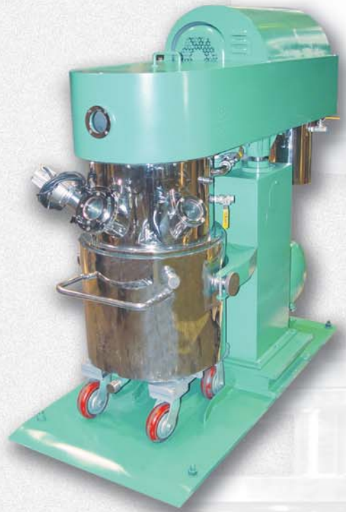
50 Liter Double Planetary Mixer supplied for the manufacture of Conductive Epoxies
